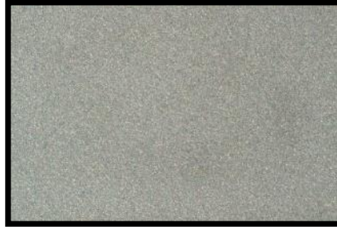
Figure 12.4: Blast cleaned steel surface to Sa 2½ standard
