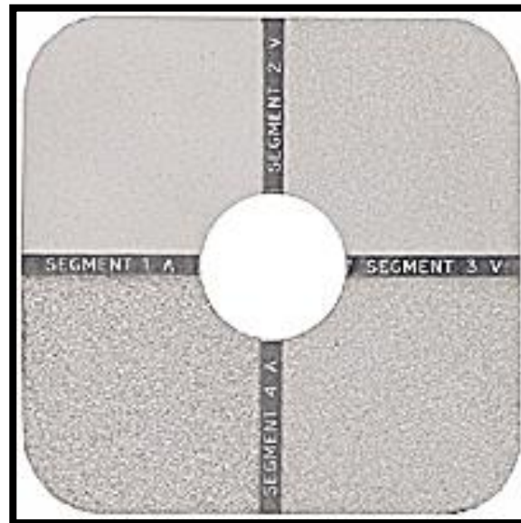
Figure 12.7: ISO comparator
